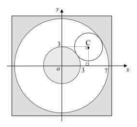
With the mechanism **fixed** in the position shown, establish the equation of the small circular disc centre C.
